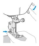
Release the button. The foot will lock in place Э level with the seam, allowing the fabric to feed.
